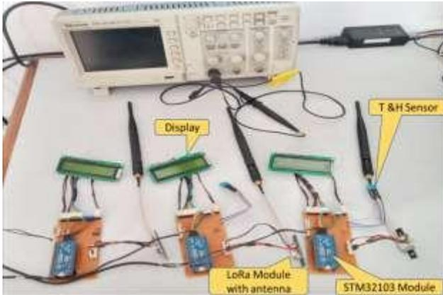
Fig. 4 LoRa system setup in lab
