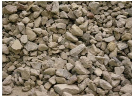
**Figure 1: Recycled concrete aggregates (RCA)**
