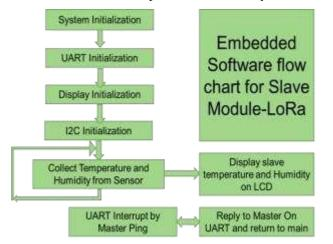
Fig.6 Slave module software flow diagram
