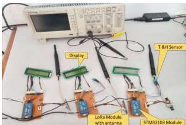
Fig. 4 LoRa system setup in lab
