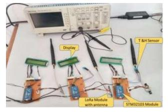
Fig. 4 LoRa system setup in lab
