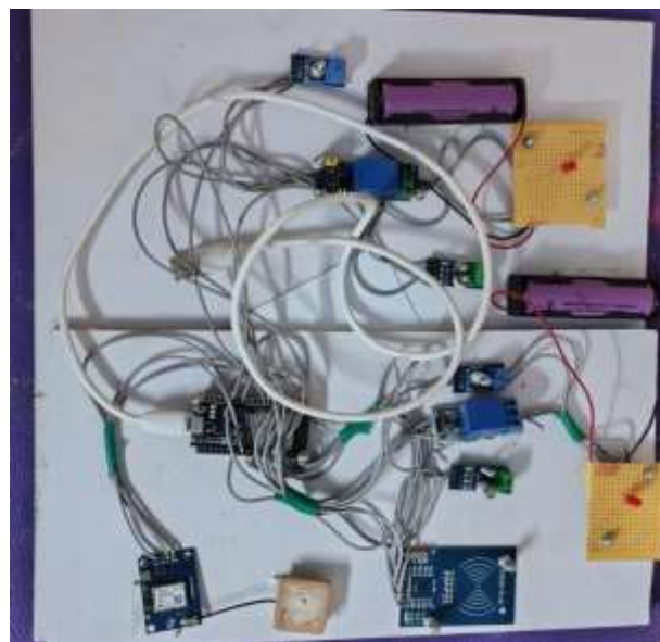
Figure 1 Overall Hardware Setup of the Proposed EV Charging System
